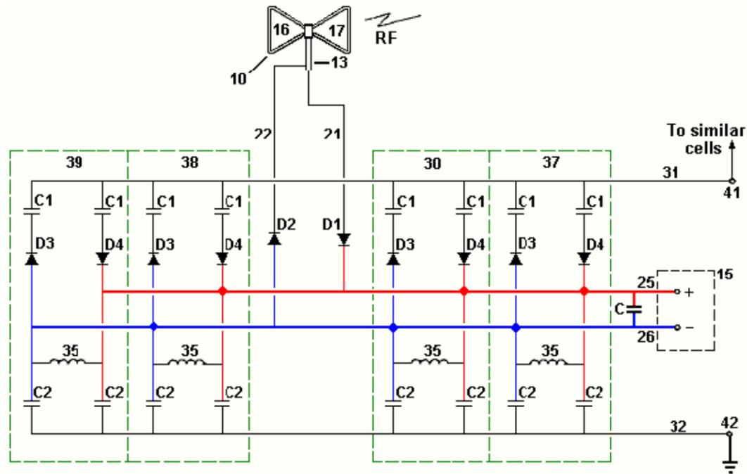
These waves are passed to the conversion circuit through a coaxial cable 13 and the DC output current of the circuit is used to power an output device 15, which may be, for example, a battery charger, DC motor, or lighting device. The circuit has no other power inputs and so has no amplifiers for boosting the RF energy.
