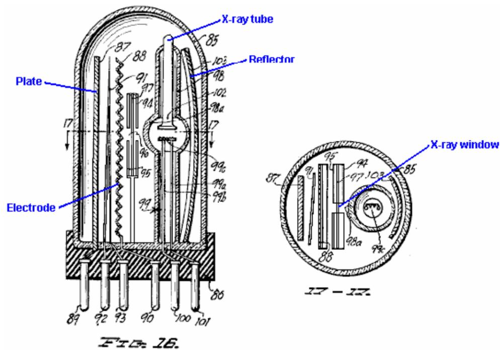
The tube of Fig.16 above, uses a different technique where an X-ray tube is used to bombard a corrugated electrode through a screen containing an X-ray window. It is thought that a brief burst of X-rays was used to trigger very short, sharp bursts of ions between the anode and cathode of the tube and these pick up extra energy with every burst.
